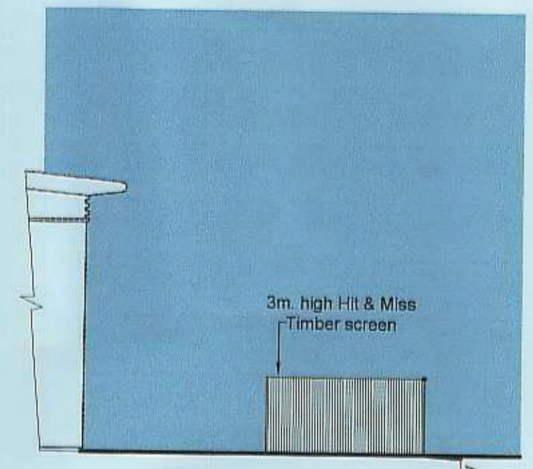
North East Elevation Service Yard Timber Screen
